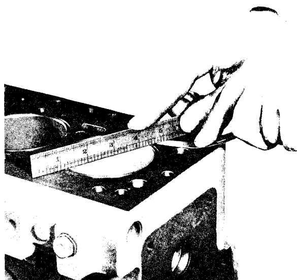
G2 Method of checking Liner protrusion.
