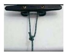
**1.** Make a loop (bowline knot) to anchor the handline and attach to cleat.
