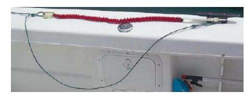
**3.** Make a small loop in the rope at the maximum stretch length of the shock absorber. Attach shock absorber to the loop.
