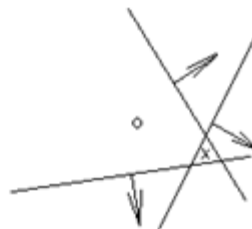
LOPs 60° apart falsely implying position x with systematic error
