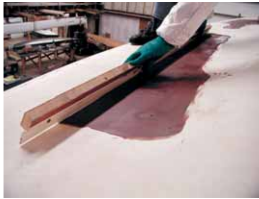
Left—I used the batten tool like a long spreader to scrape off excess mixture.
